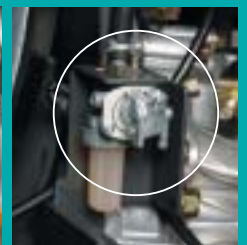
Carburetor Drain Cock* *When in use, consult operator manual and handle with care.
